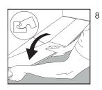
Place the short end of the plank at an angle against the previous installed plank and fold down.
