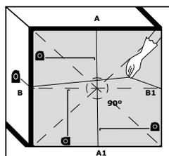
Find the center of the wall using a chalk line. Draw two symmetrical axes and use these as a starting point. Check if the intersection of the two lines forms a 90° angle. Check the wall dimension by measuring from the middle.
