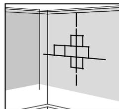
Make sure that the widths of the tiles that will be near corners are equal and bigger than 5cm (2").
