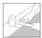
Complete first row in the same way and cut final plank of the first row to the correct length.
