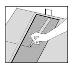
Start next row with the piece leftover (must be at least 30cm (12") long), ensuring that end joints are staggered at least 30cm (12").
