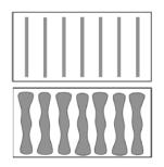
Apply the adhesive onto de substrate or back of the panel in straight vertical strings with and interval of approx. 8-10 cm.
